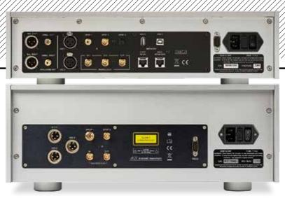
ABOVE: Transport [bottom] offers CD and downsampled SACD digital out on S/PDIF (coax and BNC) and AES (XLR). Upsampled DXD and native SACD is output on dual-AES connections. Clock in/outs are mirrored on DAC [top] with three S/PDIF ins, one USB-B, USB-A, dual-AES and LAN plus single-ended (RCA) and balanced (XLR) analogue outs
