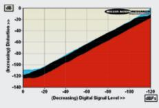
ABOVE: Distortion vs. digital signal level over a 120dB range (1kHz/24-bit, red; 1kHz/CD, black; 20kHz, blue)
